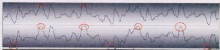
Fig. 2. The peaks circled in red are clipped.
