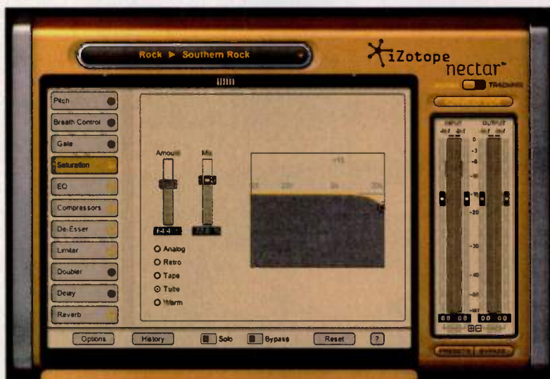
Fig. 1. iZotope Nectar adds pleasing harmonic distortion to vocal tracks to make them sound louder and bigger.
