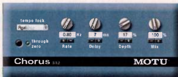
Fig. 2. Some delay-modulation plug-ins, such as MOTU Chorus, allow sufficient parameter controls for you to create the Haas effect.
