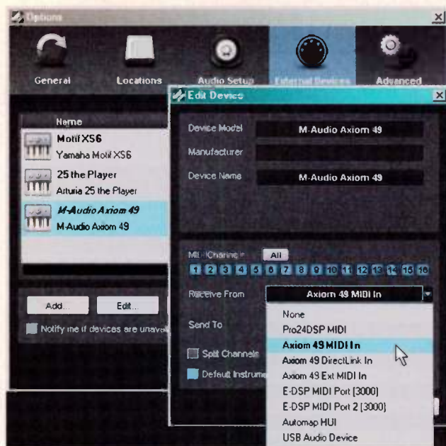
Fig. 2. In Presonus Studio One Pro, the Options menu has a tab for External Devices, where you can select your main MIDI ports from a drop-down list that shows all available MIDI devices.
