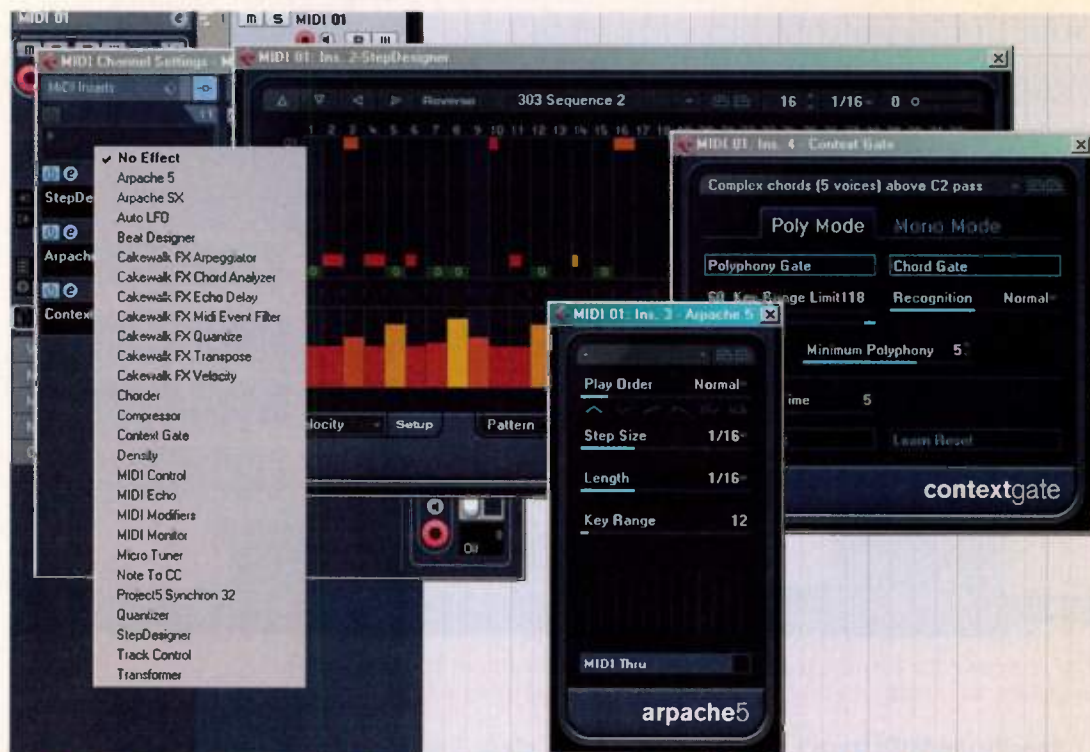
Fig. 5. This shows three Cubase MIDI FX—StepDesigner, Context Gate, and Apache 5—and a fourth is about to be selected. Note how Cakewalk's MIDI FX show up in the menu, because a wrapper has been added to Cubase that lets it recognize MIDI FX from other manufacturers.
