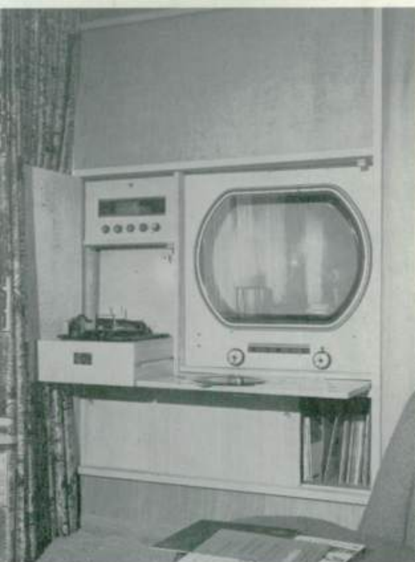
Above: Robert N. Marion, of Seattle, built this flush-wall installation in a closet. Door at left closes over the equipment, and pull-out shelf goes up to cover TV tube. Jacks at left of the TV tube are for connecting a recorder. Top section houses a bass reflex speaker; record storage at the bottom has two sliding doors
