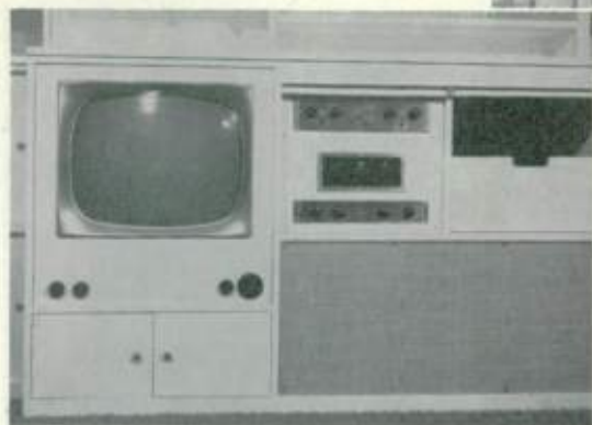
Roll-up door discloses control for 50-watt amplifier, FM-AM tuner, and drawer for record changer, with speaker below
