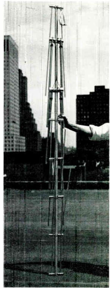
*The La Pointe Yagi is delivered as shown at the right, requiring only a few minutes to open up and clamp the rods in place. It is shown at the left mounted on a simple mast of three 5-ft. telescoping steel tubes. Maximum pickup is towards background*
