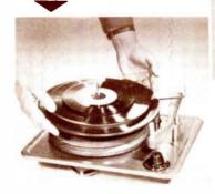
The weighted top plate levels records to obtain full advantage of the air cushion effect thus insuring against record damage.
