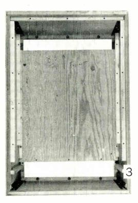
Fig. 3. This baffle must be set in place before second side is glued
