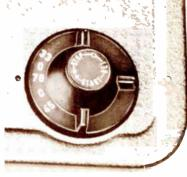
Turn the knob, and the changer will begin operating automatically. The figures on the knob refer to the speeds required by the various types of modern records.
