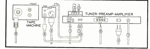
Fig. 8, below: Rear of the Bogen unit, where all the terminals are located. Fig. 9, left: An exact drawing of the terminals on the tape machine and tuner-amplifier. The changer is not shown, because it has only a power cord 4 and pickup lead 5 which plug in as shown here
