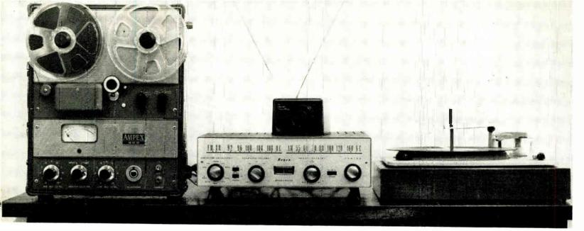
Fig. 7. Another radio-phonograph-tape system using a single unit which contains the FM-AM tuner, preamp, and amplifier
