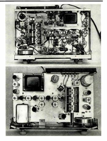
with an RF amplifier employing an AC-coupled cascode circuit. Other features include the three-gang tuning condenser on FM and AM, fly-wheel tuning, piston-type trimmers, and a goldplated escutcheon. Tubes are: 6BS8 cascode FM RF amplifier,
