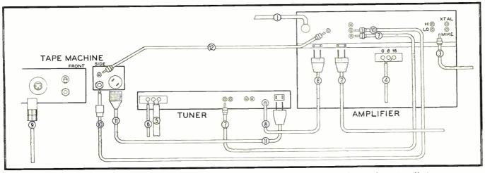
Fig. 4. Here are all the connections, just 12 in number, required for a complete hi-fi radio-phonograph-tape installation
