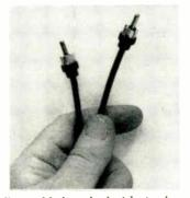
Fig. 5. Made-up lead with pin plugs Fig. 6. Terminals on the recorder
