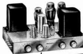
Delivers deluxe Hi-Fi sound. Includes built-in preamp; inputs for magnetic phono, mike, recorder and tuner; record compensator; bass and treble controls, etc. Response: ± 1 db, 20-20,000 cps. Distortion: 1% at 20 watts. Outputs: 4, 8, 16, 500 ohms. Chrome-plated chassis, 7 x 13 x 8 1/4". With all parts, tubes and easy instructions. Shpg. wt., 20 lbs.
