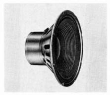
usable as a woofer or full-range speaker, has been introduced by Oxford. The speaker has a 3½-lb. Alnico V magnet, 3-inch diameter voice coil, built-in heat sink and rear vent for air relief, according to the company. A larger model, 15U10, is a 15" speaker with the same specifications.
