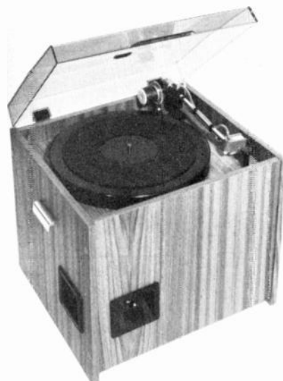
THE SEMI-PROFESSIONAL record cleaning machine by Keith Monks (Audio), Hampshire, England, removes grease and hardened sludge and loosens embedded grit with a cleaning solution and then "vacuums" the record dry. Suggested retail price for the machine is $695.
