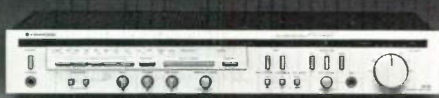
KR-80 Slimline DC Receiver. 27 Watts per channel, min. RMS at 8 ohms from 20 Hz to 20 kHz with less than 0.05% Total Harmonic Distortion; voltage synthesizer tuner with digital readout; memory preselects; auto scan; LED power indicators.
