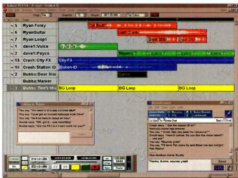
Typical Rocket Network session using Steinberg Cubase. In addition to the real-time exchanges of audio files and session data, dialog boxes at lower screen allow communication between participants in remote locations.
