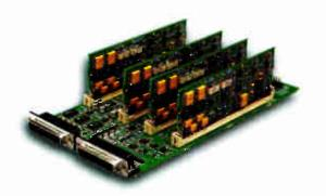
Includes Cat. No. 548 Analog Option Card for 5.1, stereo, and mono outputs to feed three separate monitor systems. The DP570D provides digital only outputs.
