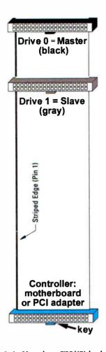
Figure 1: An 80-conductor EIDE/ATA hard drive data cable uses 40-pin connectors, and while pin-compatible with 40-conductor cables, it is not performance-compatible. Also notice that Master and Slave locations are position-specific. (For the corresponding basic jumper options, see Figure 2.)
