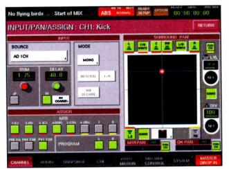
The Input/Pan/Assign screen offers fast access to essential functions.
