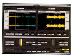
Figure 1: The newest version of Spark features a dedicated crossfode editing window for working on both ends of the waveform.
