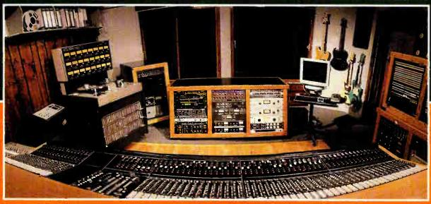
64 CHANNEL API LEGACY CONSOLE 12 CHANNEL NEVE SIDECAR BOTH WITH HEVE FLYING FADERS STUDER ABOO TWO INCH AMPEX ATR 102 HALF INCH 32 I/O PROTOOLS MIX PLUS SYSTEM ATC 150 SPEAKERS #MT 140 PLATE BEVERB TELEFUNKEN U47 NEUMANN M49
