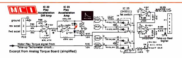
Figure 2: Portion of MCI analog torque board circuit that details how the Play Acceleration signal is mixed with the reel-motar Tachometer signal (at the junction of R97 and R46).
