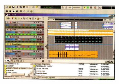
Sonar's Track view with Loop Explorer. This is the main working window in Sonar. From here, virtually all recording, editing and arranging can be done. You can also draw volume, panning and effects envelopes. The Loop Explorer on the bottom is for real-time loop auditioning. To add a loop to a project, simply double-click.
