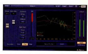
x-Noise intelligently learns from a section of naise and then applies a broadband noise reduction to eliminate background noise from a source.
