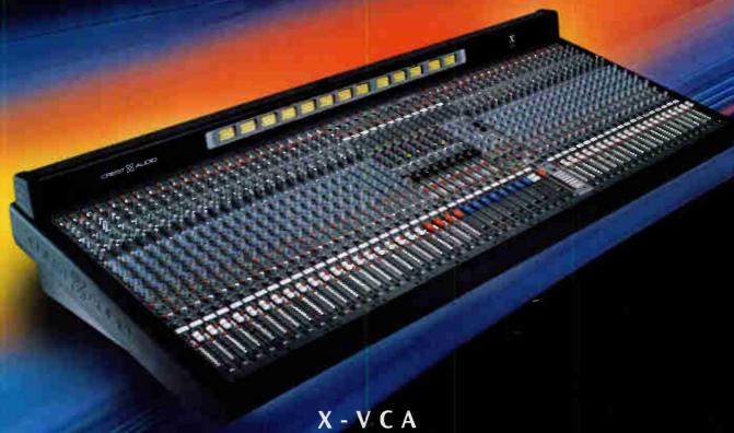
The X-VCA was designed to satisfy the most discriminating Front-of-House mixing engineer with superior sound quality at every level and a feature set generally found on more expensive consoles. X-VCA is designed for experienced operators requiring the most sophisticated level of performance. Featuring superior VCA performance (Noise/Distortion), the X-VCA uses the finest "THAT" brand VCA elements.
