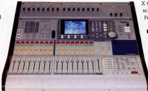
24-channel TDIF I/O and two expansion slots for DM-24-compatible I/O cards. Each of the 32 channels offers 4-band parametric EQ and dynamics, 16 buses and eight aux buses. There are four stereo effects or two 8-in/8-out surround effects.
