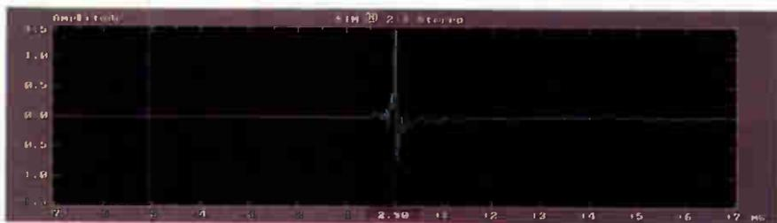
Fig. 1: HD-1's on-axis impulse response, without screen
