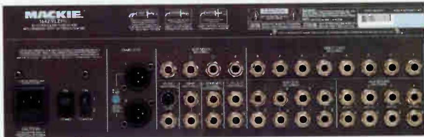
An example of good pin-1 implementation: Small touches, like Mackie's use of all-metal 1/4-inch jacks and steel rear panel on this 1642-VLZ PRO mixer, help guard against noise—creating an electrical "Firewall."
