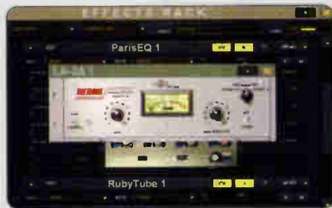
Speaking of plug-ins, the Digital X Bus is the only digital mixer in the world that runs Windows VST plug-ins internally. It supports many of the popular plug-ins from manufacturers such as Waves, Universal Audio, IK Multimedia, and Antares, plus a bunch more—and the plug-in windows are displayed right on the Digital X Bus' built-in screens.
