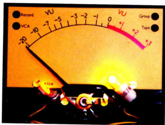
Figure 2: An SSL console meter with clear protective cover removed to access the lamps. At right, the incorrect Type 7387 bulb is installed (for comparison purposes); at left is an LED replacement.
