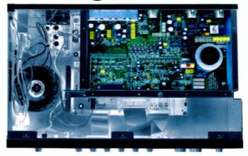
Silence is golden: At the start of the signal flow, a specially custom-wound choke is employed to ensure optimum rejection of common mode noise with zero colouration of the signal.
