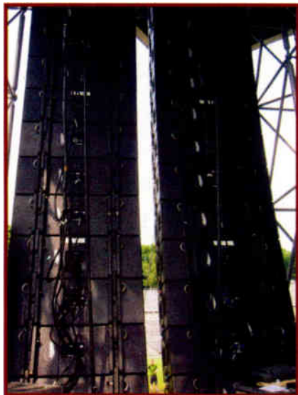
Dave Rat developed this unique P.A. structure: dual L-Acoustics V-DOSC line arrays flown side by side.
