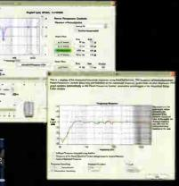
On screen, GLM software uses its *Interactive Response Editor* to give visual indication, loudspeaker-by-loudspeaker, of exactly what the response of each loudspeaker is.
