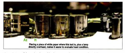
Figure 1: Four of the six heads used by the RE-301. The tape moves from left to right, starting with the erase and record, followed by two playback heads.
