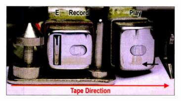
Figure 2: Two of the three Echoplex heads clearly show signs of wear, although not as extreme as the Roland Space Echo heads in Fig. 1. To the left is the combo erase/ record head, mounted on a slider to increase the distonce between it and the play head to the right.
