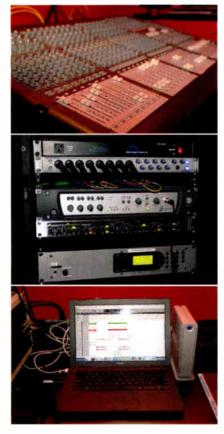
LiVE's signal flow, from top: the Mackie Onyx 80 Series console, the rack/interfaces/live-to-air streaming box and then to the mobile Pro Tools LE Mac recording setup.
