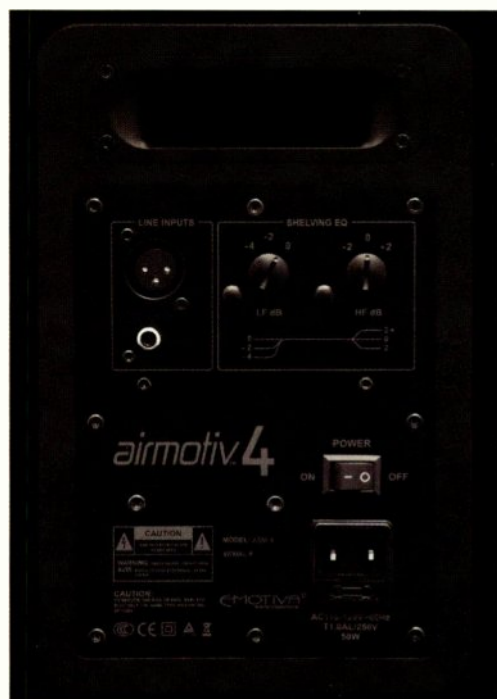
Fig. 1: The airmotiv 4's rear panel houses equalization facilities, power connections and switch, and both balanced and unbalanced inputs.
