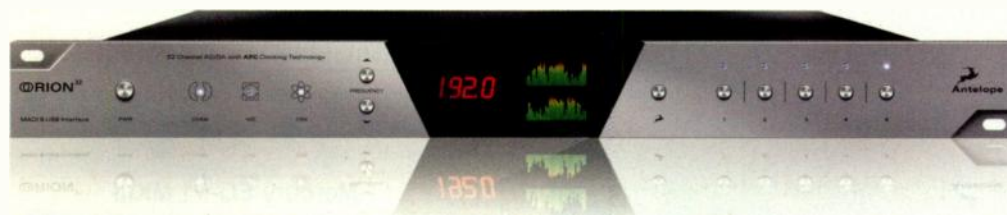
The Antelope Audio Orion 32 offers USB, MADI, ADAT and S/PDIF I/O
