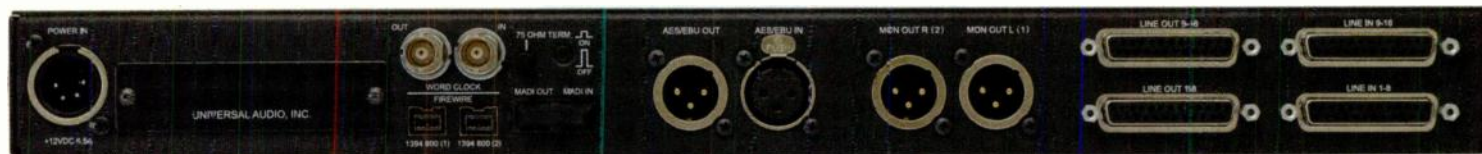
The Apollo 16's back panel includes word clock, MADI, analog, AES/EBU and FireWire 800 I/O.
