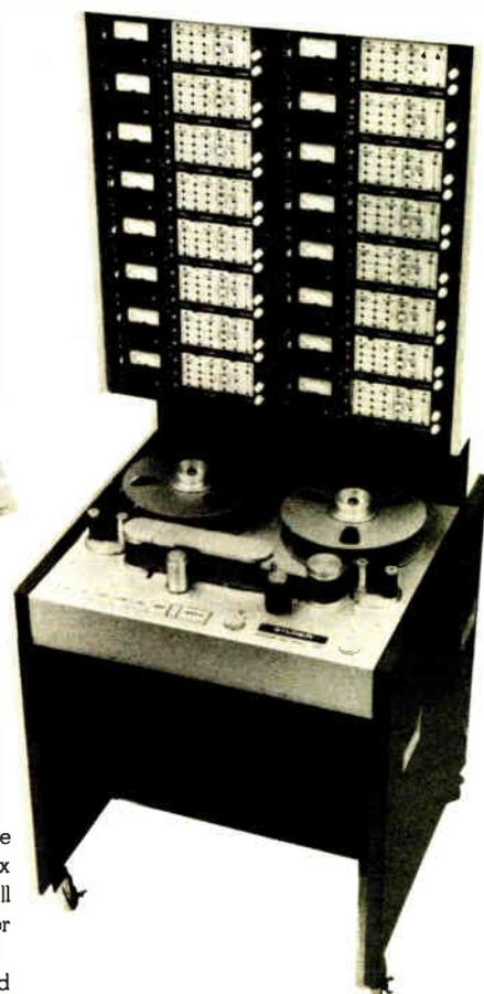
one of the first multi-track recorder manufacturers to use the I/O channel module, which contained the meter drive amplifier and the record and playback, plus sync adjustments in one interchangeable unit. The A80 MKI came in 4-8-16 track configurations. Though still very much in demand in the 16 track configuration, the A80 MKI has been replaced by the A80 MKII and the A800.
