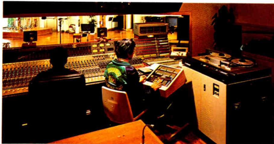
*Engineers at Tokyo's Toshiba-EMI Records studio work on a digital session with the label's Mitsubishi X-800 multitrack.*
