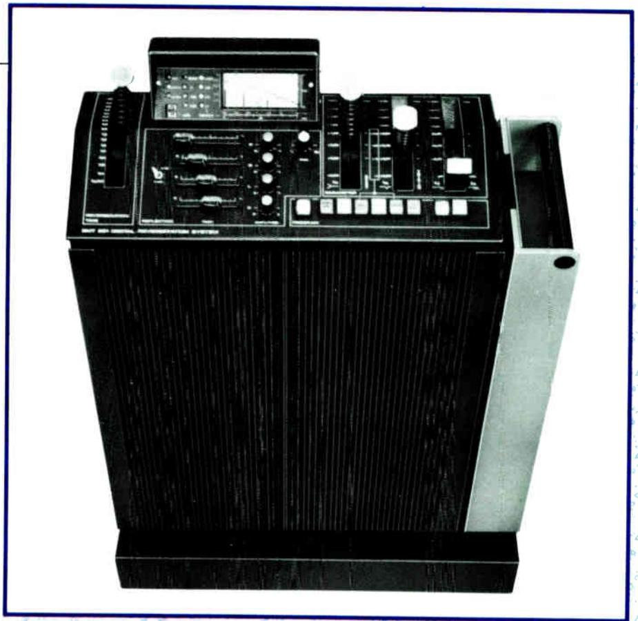
converted to analog and scaled with analog multipliers, summed together, and output. It was supposed to be an improvement on the multiple-head tape idea, but the design's single feedback path made regular iterations which were quite audible. A number of smaller circulating loops sounded better, but suddenly there was a lot more digital arithmetic and memory access needed, and the hardware got more complex.
