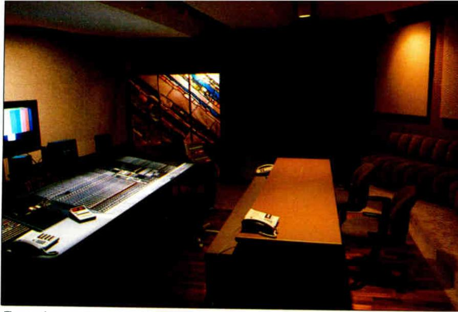
*Control room B at New York City post-production house Sync Sound. The clean, uncluttered design is achieved by locating multitracks and video decks in a centralized machine room nearby.*
