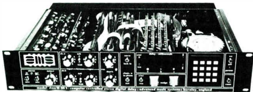
The AMS Model dmx 15-80S was the first digital delay to include sampling capability.
