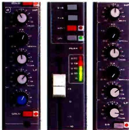
**DETAIL:** Auxiliary modules have three band EQ with variable Mid frequency for more usable, functional outputs.
