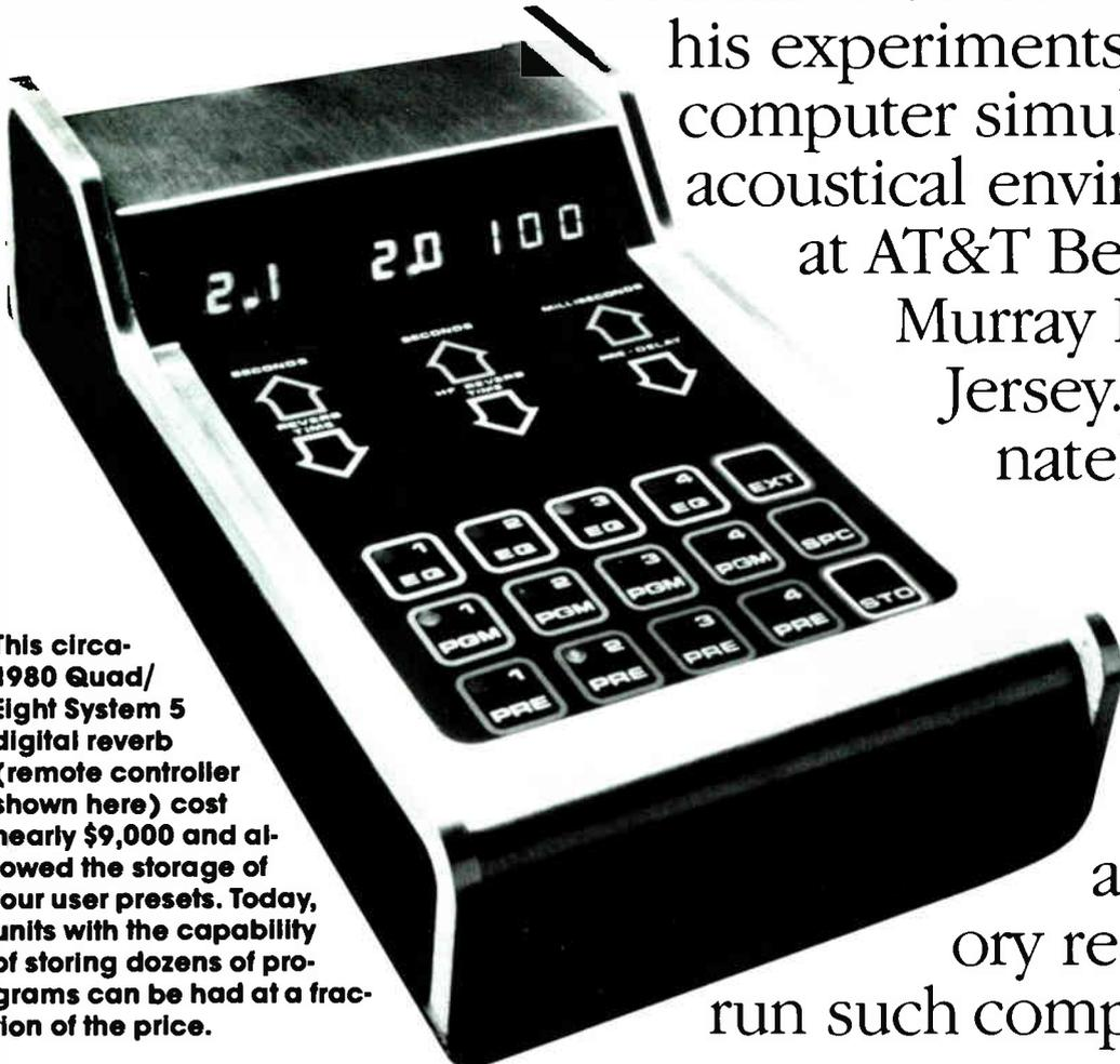
This circa-1980 Quad/Eight System 5 digital reverb (remote controller shown here) cost nearly \$9,000 and allowed the storage of four user presets. Today, units with the capability of storing dozens of programs can be had at a fraction of the price.
