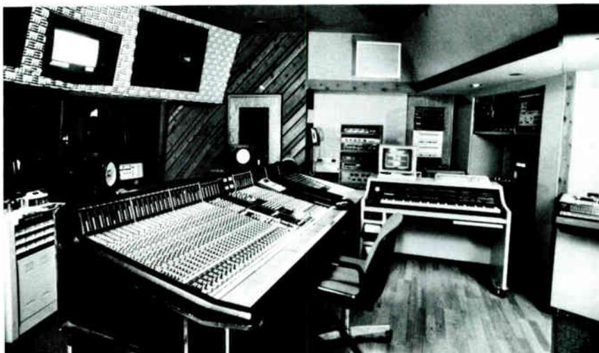
"The Finishing Suite:" SSL with Total Recall mix automation, 5 machine synchronization, 24/48 track to 1" video mixing.
