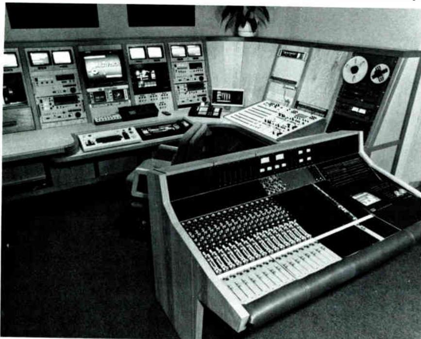
**At the Multivision video facility, this custom, automated audio console and the AMS Audiofile are controlled by time code on the master video tape. Digital multi-channel audio—including SFX off CD—mix down directly onto the one-inch master.**
