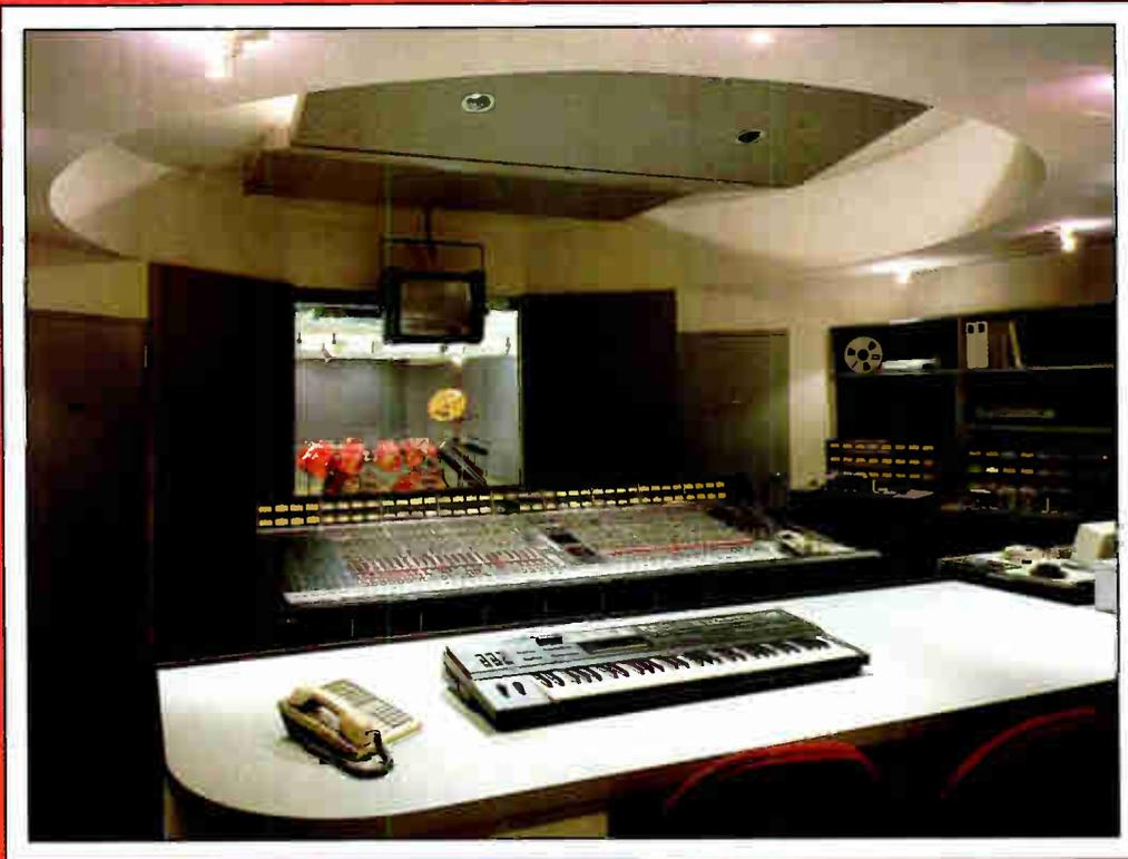
Acoustically designed by Vin Gizzi of Benchmark Associates, the spacious Room 1 at Power Play Studios in Long Island City, NY boasts an SSE 4000 E console, two MCI JH-24 recorders and a Sany PCM 3202 2-track digital machine. Out-board equipment includes a Lexicon 224 XL digital effects processor, an AMS DMX 15-80S digital delay and an AMS RMX 16 digital reverb. Power Play has hosted recent recording projects for MCA, Chrysalis and Island Records. Photo by David Bevan.
