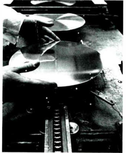
**Polished aluminum discs are loaded onto a conveyor for transport to a lacquer coating machine.**
