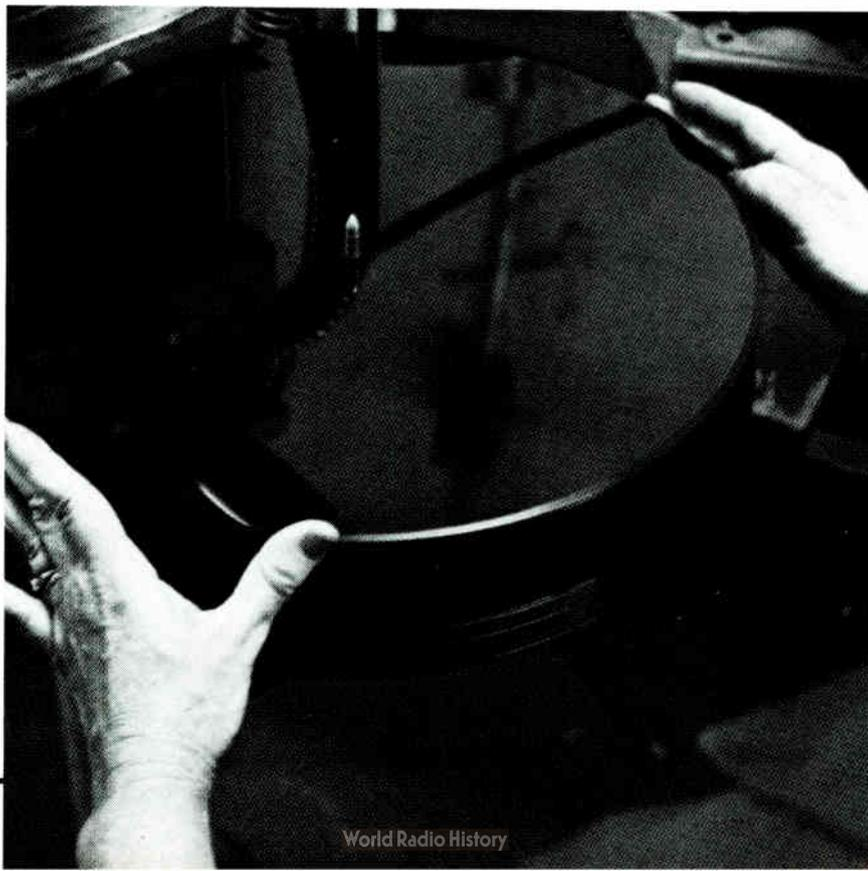
The highest grade of flat, smooth aluminum and a proprietary lacquer formulation are skillfully combined to produce the finest recording blank obtainable.
