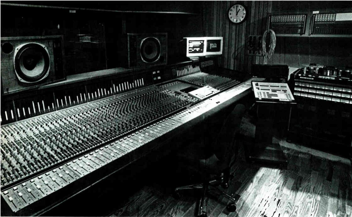
cility who backed out on it, so it was ready for us—we ordered it in December and got it in January. It has a 4000E series frame, but the electronics are 90% G series. It's a 56 frame loaded with 48 modules, and we got the plasma display. We're installing the Bernoulli [data storage] drives, and bought five remote tape transport controllers with it. Along with the quality of the new EQ, we chose SSL for its ergonomics, plus its compatibility with other studios."
