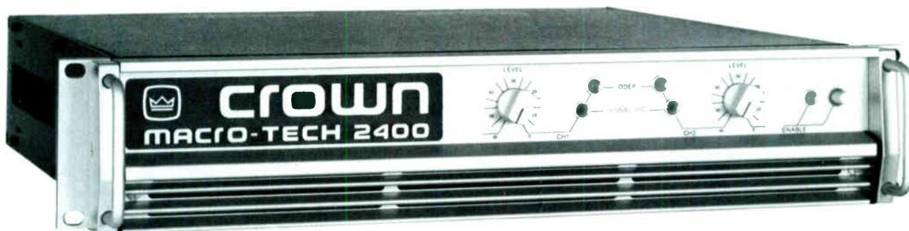
the temperature of the power transformers. If temperatures rise too high, the amp shuts down until it cools to a safe temperature, at which time it automatically becomes operational.
