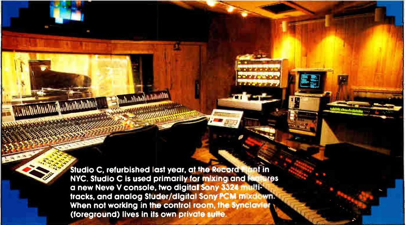
Studio C, refurbished last year, at the Record Plant in NYC. Studio C is used primarily for mixing and features a new Neve V console, two digital Sony 3324 multi-tracks, and analog Studer/digital Sony PCM mixdown. When not working in the control room, the Synclavier (foreground) lives in its own private suite.
