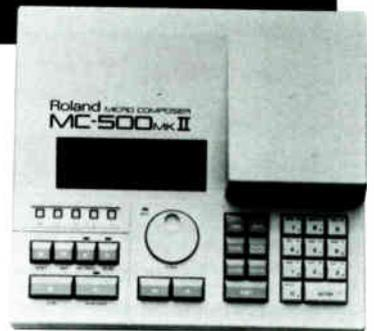
capacity is 100,000 events, with additional storage via the unit's built-in 3.5-inch floppy drive. Another feature is the MC-500 MkII's two independent MIDI outputs for controlling up to 32 MIDI channels simultaneously.
