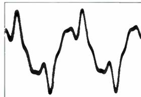
*This is what a typical filter chain does to a 2.5kHz square wave. Think what it would do to Beethoven. Or to Rock'n'roll.*
