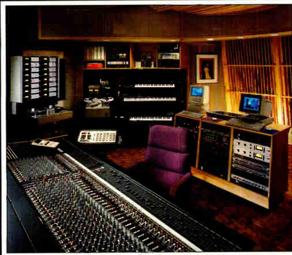
Originally built in 1978 by John Storyk, Horizon Studio was rebuilt late last year by co-owner Vic Steffens with acoustical design assistance from Storyk. The centerpiece of the control room is a 44 x 24 Allen & Heath Sigma console with built-in mute automation run from either a Mac or an Atari ST. The facility is used for both live and MIDI productions, making use of an adjacent 875 square-foot live room with c 14-foot ceiling and a full MIDI facility in the control room. Photo: Tracey Kroll
