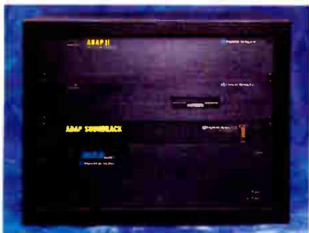
for Analog to Digital Audio Processor. In short, ADAP is a digital mastering device and audio work station, a 16 bit stereo sampler, a visual non-destructive sound editor with sample precise accuracy, a MIDI module, a SMPTE trigger, full EDL (Edit Decision List), a cue system and much more.
