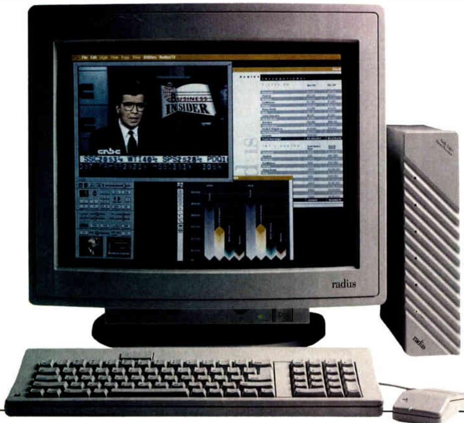
**Above:** The “pocket accessor”, Paul Brainerd’s vision of the computer of the future. **Left:** Radius TV features a video processing engine, an external audio/video input processor and television tuner that allow display and digitizing of live 16-bit video images at 30 fps on Mac II computers.
