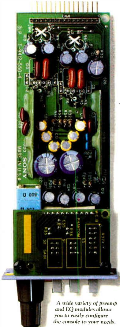
A wide variety of preamp and EQ modules allows you to easily configure the console to your needs.
