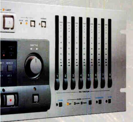
Take punching-in and out, for example. You have three easy ways to do it. You can punch-in and out of single tracks on the fly. Just hit the track button at the punch-in point. Hit it again to punch-out. You can use the optional foot switch, if you like.
