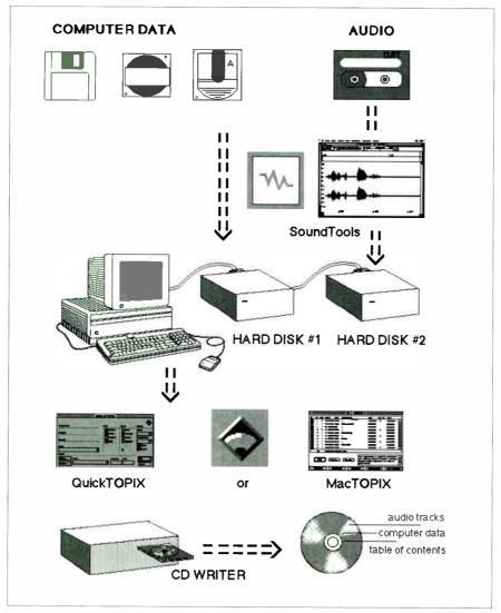
Figure 2: Flow chart showing the master-making process for a mixed-mode CD-ROM
