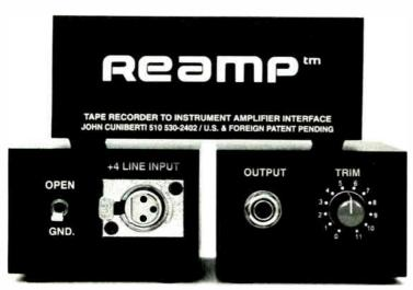
REAMP is about the size and shape of the popular Countryman direct box. Because it is passive, there are no batteries to change, and it is RF-protected. On the input side is a ground lift switch and a female XLR +4dBu connector in which to plug your tape track output. On the output side is a volume trim pot (yes, it goes up to 11) and a 1/-inch jack for connection to an amp.
