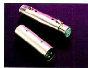
Switchcraft® offers a complete line of adapters including the 3-contact female to female, #389 (with Switchcraft A3F inserts at both ends) and the 3-pin male. #390 (with Switchcraft A3M inserts at both ends). Both the #389 (shown at top of photo) and the #390 (shown at bottom of photo) have pre-wired contacts. The female version has a polarizing boss; the male version has a polarizing groove.
