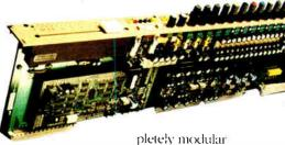
design allowing any of the five input module types to be placed anywhere in the compact (32-inch frontto-back) frame. Input modules may be single or dual and feature 4-band parametric EQ plus high- and lowpass filters and switched inserts. The F-Type may be specified with up to 12 subgroups, 24 matrix groups and 16 aux buses, and integral I/O metering eliminates the need for a meter bridge. The F-type uses the same automation as
