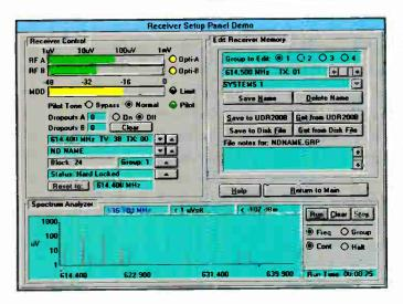
The UDR200B receiver is supplied with LecNet<sup>TM</sup> software to run under the Windows® operating system. The control panel for an individual receiver shown here includes indicators of present receiver settings and levels, an edit section to make changes, store and retrieve files, and a spectrum analyzer section that provides a spectral plot of the tuning range of the receiver.
