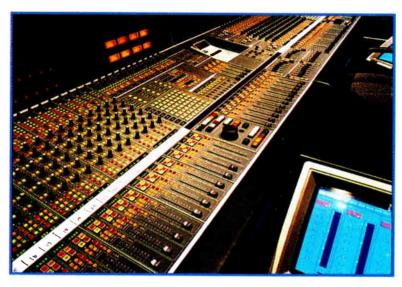
to any experienced mixer or rerecording engineer. Software-controllable functions are handled via a high-res, touch-sensitive VDU at each of the music, effects and dialog mixing stations (assuming a conventional three-person console layout). Multiple pages on the MPC's Interactive Touchscreen Interface (ITI) are quickly accessed from the menu bar located at the top of the display.
