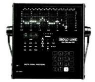
1/3-1/6 and 1/12th Octave Analysis = 1/4dB Accuracy = 85dB Window = SPL Flat, A, C, User = RT-60 = Speaker Timing = 30 Non-Volatile = Memories = RS232 Windows Interface = NC Measurements Retail \$1,579 Call for Contractor Price
