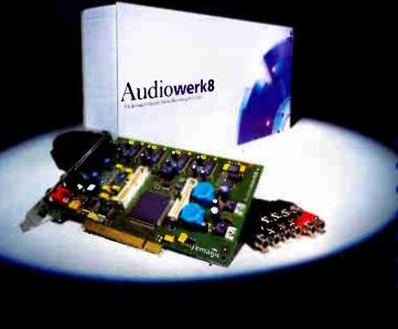
Introducing Audiowerk8, the affordable 8 Channel Digital Audio Recording PCI Card featuring:
