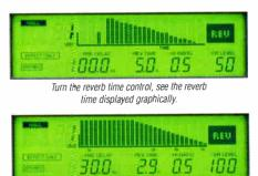
Turn the HI-RATIO control, the REV500 instantly shows high frequency decay.
