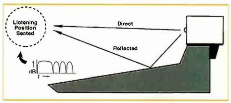
Figure 5: Reflections interact with listener (causing comb filtering) when speaker is placed on console top.
