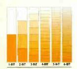
Every bit you add doubles the resolution of a digital recarder Compared & 16-bit formats, ADAT Type II's non-compressed, linear 20-bit recording offers a wider dynamic range, less quantization distortion at low levels, mare headroom and even lower noise. Result: detailed, full-spectrum audio fidelity that far exceeds the quality of any analog recorder
