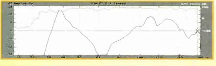
Figure 1: Bass response of speaker placed along the short wall,
