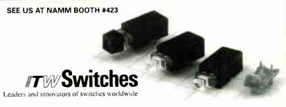
Requiring minimal PC board space, the UltraLite Series 39-7 minipush-button switch provides clear, bright LED status indication and a logic-level rating of 5 mA, 5V dc typical. The switch, which offers maintained or momentary actions, is only 0.25" high and 0.30" wide. LEDs come in three colors: red, yellow, and green.
