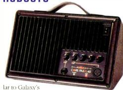
lar to Galaxy's HOT SPOT), the 13-pound system is capable of 114 dB SPL and features a frequency response of 150-15k Hz. XLR and ½-inch inputs have individual volume controls, and an automatic gain control circuit adjusts for instrument, mic and line inputs. The unit also includes a 3-band EQ, a built-in compressor to prevent clipping and a post-EQ RCA output, Price: \$399.95.
