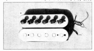
the bottom hole for the exit of the beginning wire of the coil
