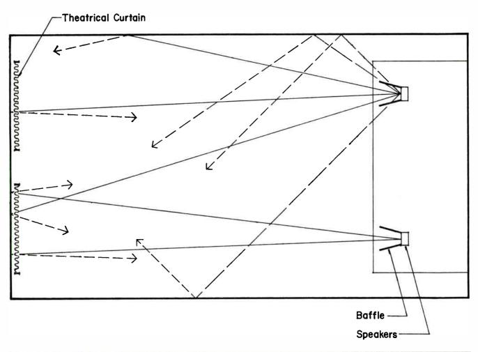
Theatrical curtains can significantly reduce reflections when deployed over fairly large areas, while smaller baffles around loudspeakers suppress unwanted reflections at the source.
