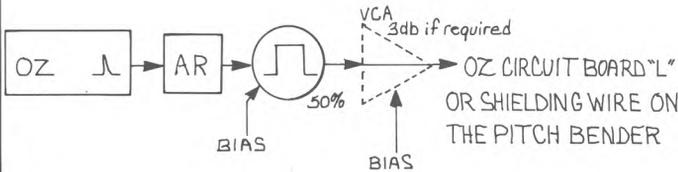
If an amplified waveform from a VCO is used a variety of voltage controlled vibrato effects may be produced.
