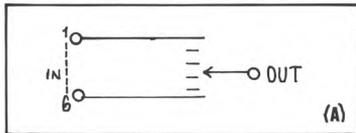
Note that this is a six-position switch. This would accommodate square, sawtooth, triangle, sine, modulated pulse, and noise. This switch, being a passive unit, is bi-directional; that is, inputs could be outputs and vice-versa. I built two such switches, and they serve me very well.
