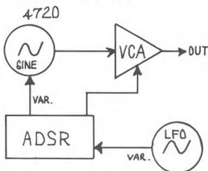
VCO pitch should be set high. Increase LFO output to trigger ADSR at proper rate. Set ADSR variable output to obtain proper frequency change. Work with one hand on the initial pitch knob and the other on the ADSR attack knob. Decreasing attack time gives a warble effect. Pressing the manual trigger stops sound well.
