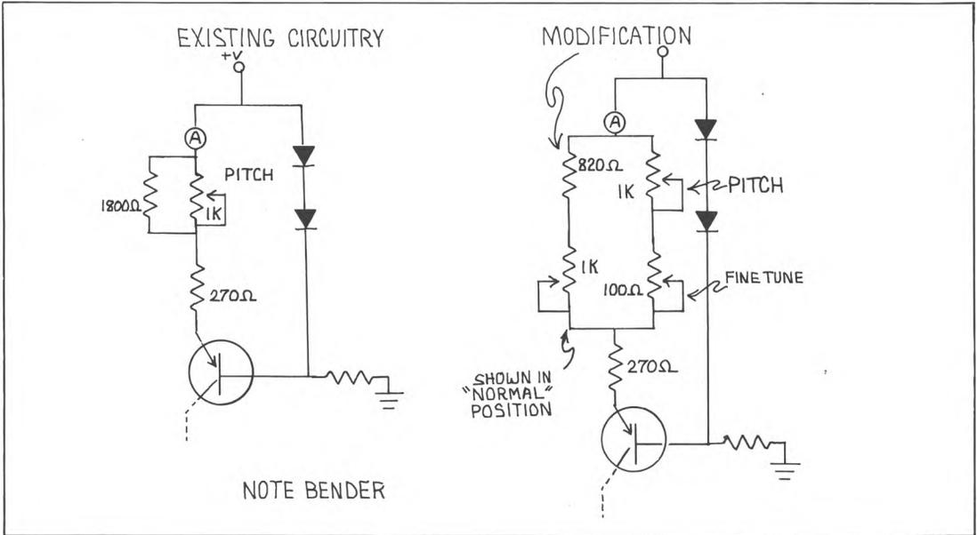
A modification of the Sample and Hold circuit in the Keyboard Controller of my synthesizer provides a note bender. This effect is used extensively by Jan Hammer (with Jeff Beck), Patrick Moraz (Yes) and Roger Powell (Utopia). It is used the same way as a guitarist bends a note.
