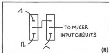
I mounted these switches just below the Pulse Width control knob, and included appropriate labels. One switch selects either the "hard" or "soft" waveforms. When wiring these switches, wire directly to the proper point on the output jacks of the oscillators. Here is versatility again, since the oscillators may be mixed, yet each output is separately available.
