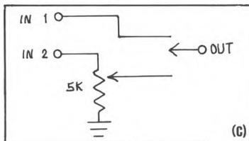
Patching the variable output into (1) and the fixed output into (2) allows for two totally variable outputs which are instantly and exactly repeatable.
