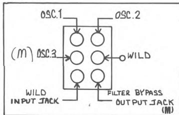
We still have one problem. How do we select which waveform goes into the mixer? This will require some modification to the oscillator panels. A simple Or type of switching is used, and constructed from two SPDT switches. Each oscillator will require one such switching circuit.
