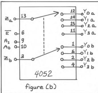
and whereas the 4051 was an electronic equivalent of a Single Pole Eight Throw switch, the 4052 is like a Double Pole
