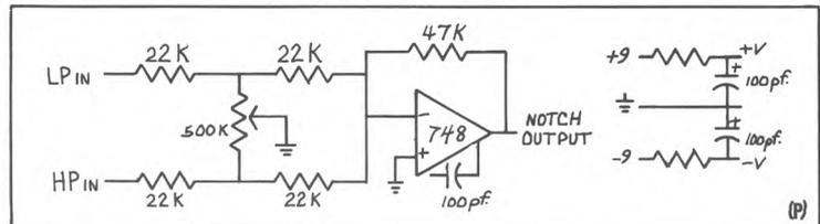
This circuit produces an output that is continuously variable from lowpass through notch to high pass. I must admit I have found this tuning ability to be of little use, so if it is not desired simply remove the 500K pot and replace the two 22K resistors in each leg with one 47K resistor.
