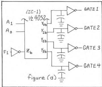
This is a little S/H in its own right - but it doesn't hold an analog voltage, only a "1" (output high) or "0" (output low).
