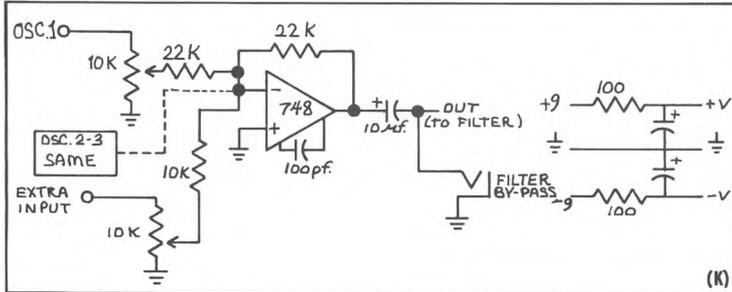
Its action is such that if nothing is inserted, terminal 2 is connected to terminal 3. Terminal 1 is ground. In use, terminal 2 will make no contact with anything inserted in the jack, while terminal 3 will contact the tip of the plug. We can use this as shown below.
