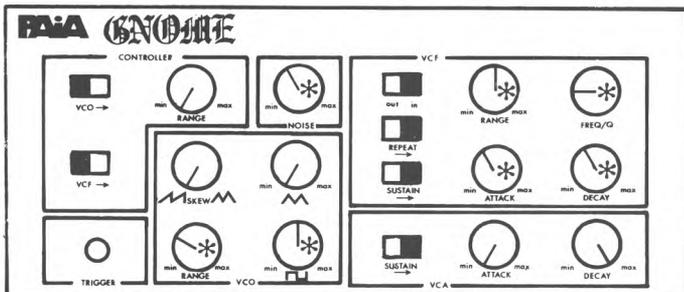
Set VCF controls for the whirling blades. Mix NOISE and VCO for proper amounts of blade noise and engine sound. Set VCO Range for subsonic "putting" of engine.
