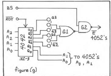
The 4042 Quad Latch is an old friend - here we're reusing it to latch the computer's 4 least significant address bits at the same time that data is put out to the D/A (the RDY line on this card is connected the same as the corresponding line on the D/A).
