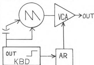
Obviously a simple patch, the AR can be set to any standard envelope, filters can be added, etc. The capacitor (from the 2720-7 Power Supply) acts as a differentiator, and when added to the straight control voltage produces a spike on the normal change. The effect increases as the interval between notes increases, and an interesting effect results when
