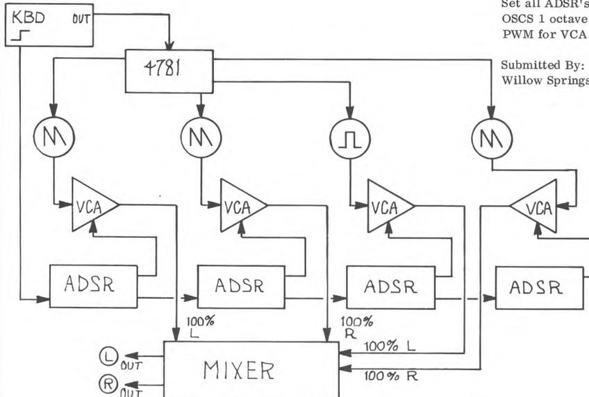
Set all ADSR's for full attack. Offset OSCS 1 octave apart. Try substituting PWM for VCA or VCF for VCA.
