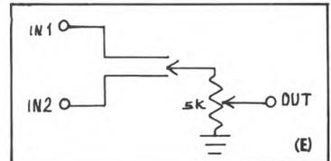
One important thing to note. Each of these circuits require a ground reference. I built two of the audio switches and two of the control switches in the same box. I always use shielded cable, so all of the grounds (including audio) can be tied in through the shield. If you build the control switches alone, it will be necessary to make provisions for a separate ground input jack.
