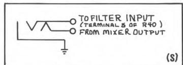
for the oscillators and 2 for the extra (or wild) input. The wild input is for adding another oscillator, noise, or cascading filters. The extra gain makes up for some signal loss. Be careful that the total input does not exceed that allowable for the filter, or distortion will result.
