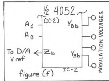
Because the modulation voltage corresponding to a given control channel is applied to the D/A only when that channel is re-freshed, you may think you will be able to hear the modulating influence as a series of steps. But you don't for the same reason that the glide doesn't appear to be a series of steps. Everything is just happening too fast.
