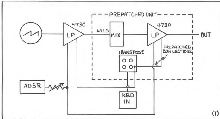
the transposer knob, and a sweep may be applied to both filters at the same time. (see figure (t).) Take note of how the keyboard voltage is prepatched into one filter and externally patched to another.
