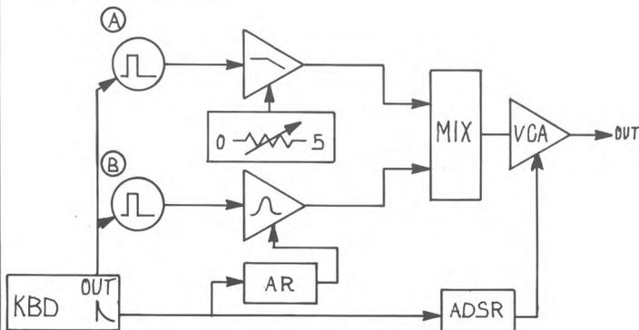
VCO B tuned one octave lower than VCO A. Both VCO outputs are narrow width pulses.
