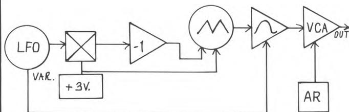
The LFO should be set to about 7 Hz., and on the output to the BPF about 4 volts. The modulation control on the Balanced Modulator is set right before the LED comes on. The 5 volt offset can be varied for different pitched cries. The BPF-Q is at about 75%. The AR is set for minimum attack and 50% release. To play just push the manual trigger and release.
