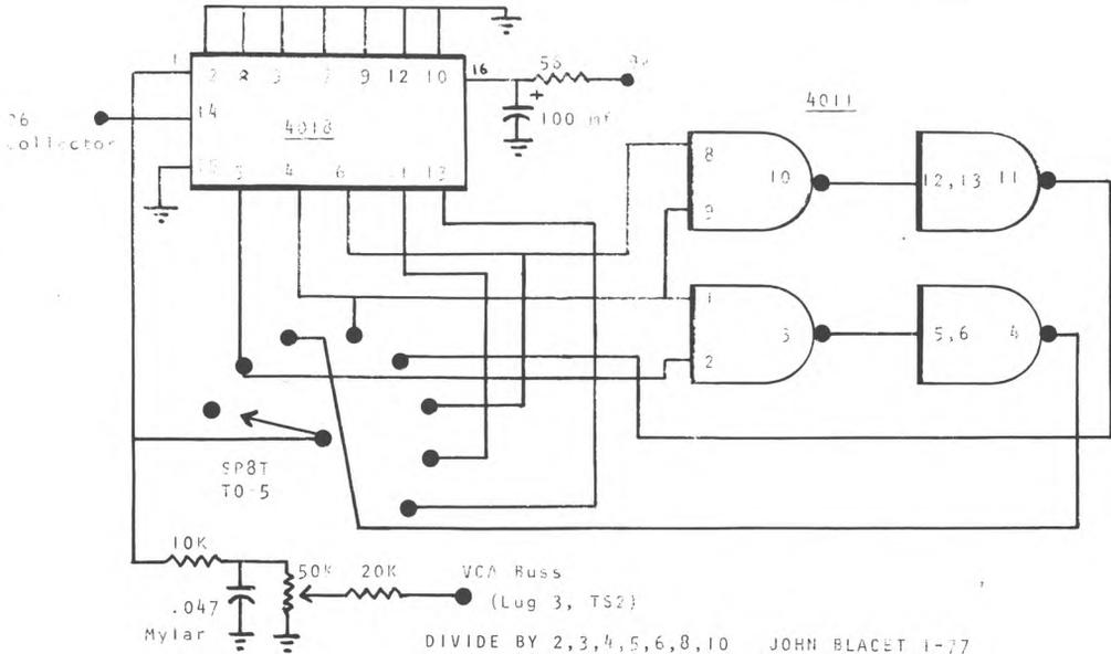
Here's the schematic for the frequency divider that I've been using with my Gnome.
