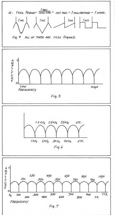
these peaks and valleys occur is a function of the delay time. The delay time is, of course, dependent on the number of stages in the delay chip (512 per side of the SAD 1024) and the clock frequency (usually from 30KHz to 500Hz).
