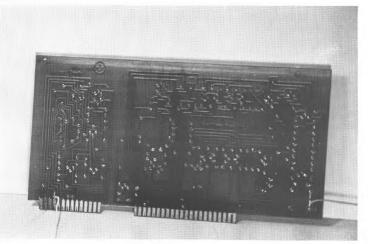
the board is the B socket section. This section consists of 22 contacts, once again designated on the circuit board from left to right as #1B through #22B. See figure 9.
