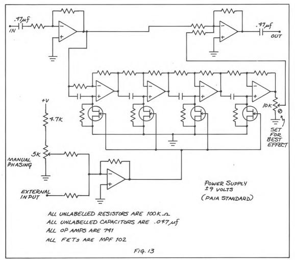
many of the popular 'pedal phasers'. Many larger units use 6, 8, even up to 12 such stages. In general, two stages produce a notch, and three are necessary for a hump.
