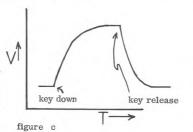
Because the glide is now on during the entire attack cycle and the Decay and Sustain portion of the transients are eliminated. Straightforward stuff, really.
