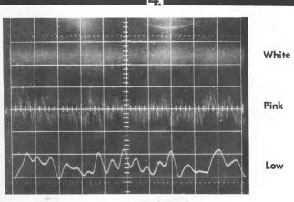
volts AC on the VTVM. See Figure 4. By the way, if your VTVM has a dB scale on it then these readings should read about -2 dB. Place the scope on J9 and 3 volts of low random noise should be seen, or .6 volts AC on the VTVM. See Figure 4.
