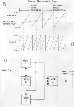
vovel sound and opening this attenuator fully slides the VCOs upwards stopping at the frequencies which will produce the second vowel sound. This timbral change should occur within the temporal space of one amplitude envelope. Using an envelope with a moderately long actack and release generally yields the best results.
