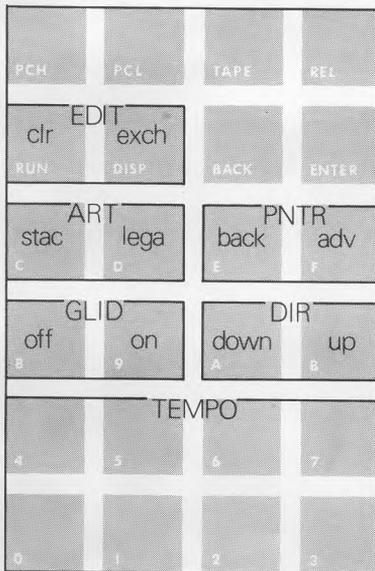
Touching the DIR:UP pad will cause the arpeggiation to change direction from down-scale to up. GLID:ON turns the glide for the arpeggiation channel on and (you guessed it) GLID:OFF turns it off.
