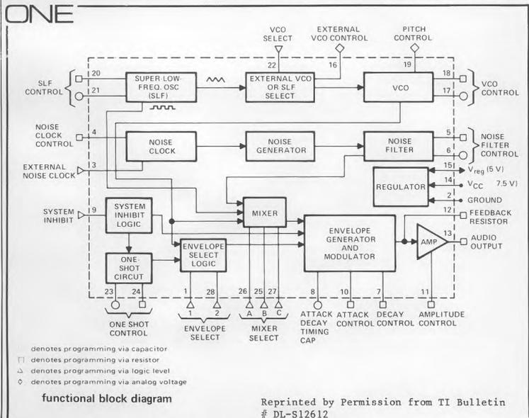
(pin 14). If a 5 volt supply is used, connect to pin 15. This pin becomes a 5 volt source when pin 14 is used as a power input. All external voltages should be sourced from pin 15.
