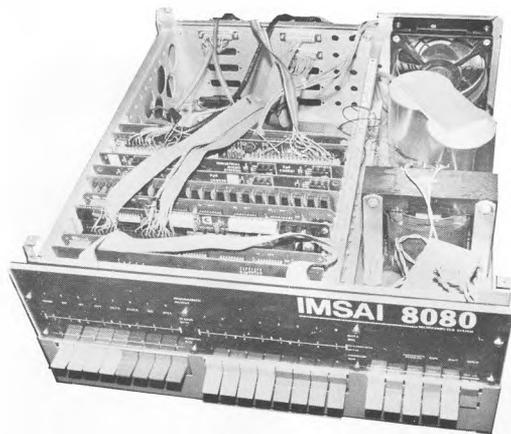
PHOTO #1 - Close up of the IMSAI's internal workings. The set of eight switches to the left function as our record switches. The LEDs above these switches served as a visual reference when calibrating the synthesizers.
