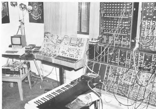
PHOTO #2 - Shown clockwise from left; IMSAI 8080, Apple II Plus with two disk drives, GBC - ITC monitor, Serge six panel custom synthesizer, Moog 55, Moog Sequencer, Moog 15 and a Polyfusion 2054 keyboard.
