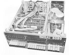
PHOTO #1 - Close up of the IMSAI's internal workings. The set of eight switches to the left function as our record switches. The LEDs above these switches served as a visual reference when calibrating the synthesizers. connectors and both phone and banana jacks to accomodate the synthesizers. Presently we are in the proccess of adapting ACT for use with the Apple.
