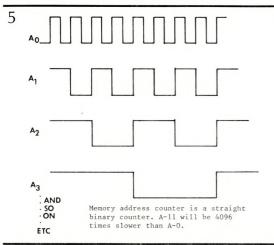
The memory address counter built around U14, U15 and U16 is checked by setting the delay program switches for maximum delay. In this condition each IC will count down the pulses by 16. The scope is then used to see that AO (address line #0 - the least significant or "fastest" counting line) through All (address line #11) have outputs of decreasing frequency.
