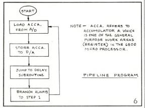
The "pipeline" flow chart is self-explanatory with the exception of the delay subroutine. A subroutine is a service routine called by another program. Upon completion of the service routine, program control is transferred back to the
