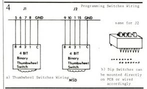
of the memory address counter, allowing delay memory length to be set anywhere from 1 to 4096 bytes. This permits the audio delay to be varied while holding the sampling rate constant. Although the use of switches provide the most convenient way to adjust the delay to the needs of the room where it is being used, the delay can also be programmed by fixed jumpers, or interfaced with external TL signals such as a microprocessor.
