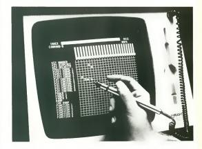
In the case of a "created" sound, a number of methods are used whereby sounds can be synthesized. One of these methods is by "drawing" a series of harmonic profiles (envelopes) each with its own character of attack and decay.
