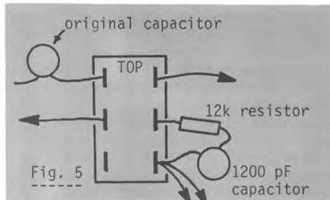
inserted into it. This will prevent the resistor from swivelling around. Also, I generally use shielded cable to make connections to the master volume pot, since this part of the amp is more likely to pick up hum than the section illustrated in figure 1.
