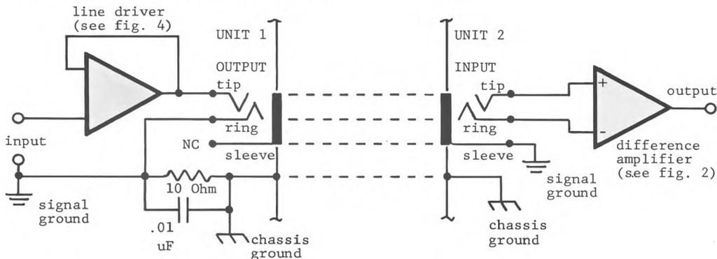
Figure 5 Interconnection between units
