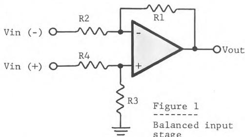
here the solutions expand (as does the cost) to two and three op amp instrumentation amplifiers. The main advantage of the more complex circuits is their equal input impedance characteristics. A characteristic not exhibited by the single op amp difference circuit, with one exception. Patience, I'm getting to it!
