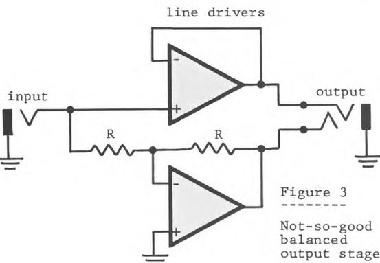
Figure 3 Not-so-good balanced output stage
