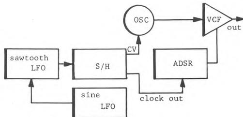
Figure 8: Sawtooth S/H with Evolving Phase
