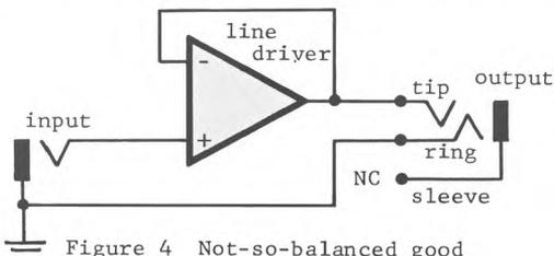
Figure 4 Not-so-balanced good output stage
