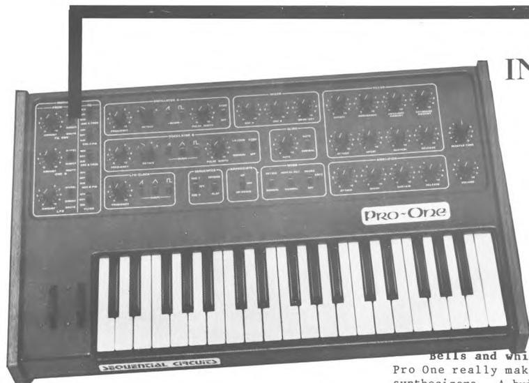
The Pro-One is a small monophonic performance synthesizer based on circuitry made famous by its polyphonic parents, the Prophet-5 and Prophet-10. The Pro incorporates many features that make it a real value in its price range. These include a 40 note sequencer function (true sequencing, not FM wave-shaping) with the ability to add rests in the program, an arpeggiator, and an external audio input for instrument treatments and processing.
